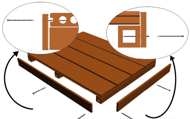
Fix the side pannel to the parallel joist or decking board.
